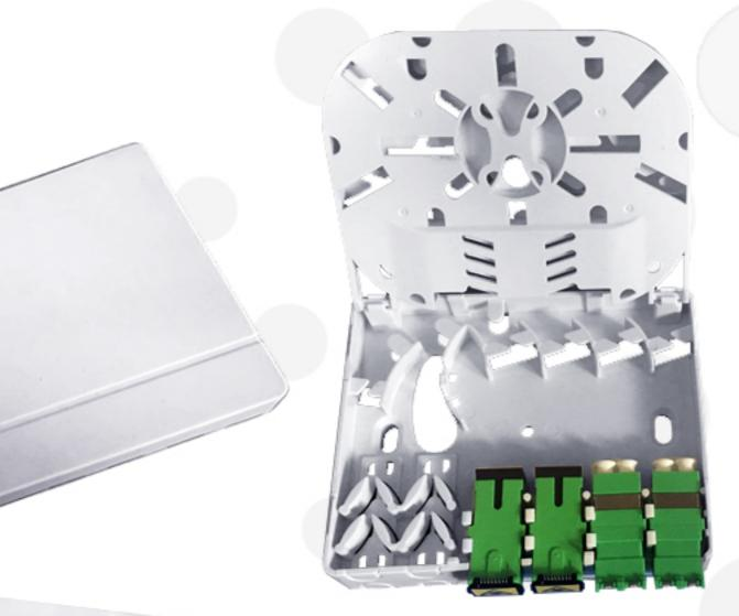
D-Connect's FTTH Fibre rosette box series fiber rossette box is able to hold up to 4 subscribers. It is used as a termination point for the drop cable to connect with patch cable in FTTH indoor application. It integrates fiber splicing, termination, storage and cable connection in one solid protection box.
