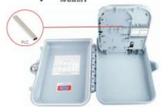
FAT-16D fiber access termination box is able to hold up to 16 subscribers. It is used as a termination point for the feeder cable to connect with drop cable in FTTx network system. It integrates fiber splicing, splitting, distribution, storage and cable connection in one solid protection box.
