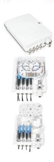
FAT-8E fiber access termination box is able to hold up to 8 subscribers. It is used as a termination point for the feeder cable to connect with drop cable in FTTx network system. It integrates fiber splicing, splitting, distribution, storage and cable connection in one solid protection box.
